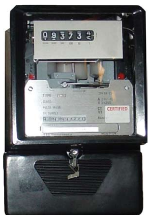
Figure 1. Electromechanical energy meter.
