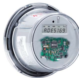
Figure 2. Solid-state electronic energy meter.
